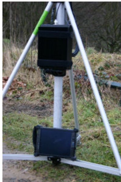
Mast-mounted MIST-RD server with a portable Tablet PC resting on the base
