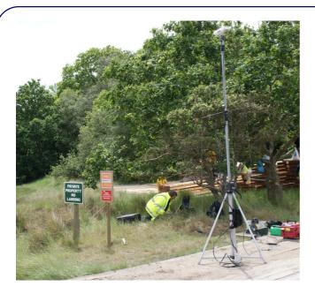
The system is designed specifically to address the issues surrounding long-range surveillance. The system is easily transported in the boot of a car; it requires no mains power or wired communications and can be deployed by a single person.
