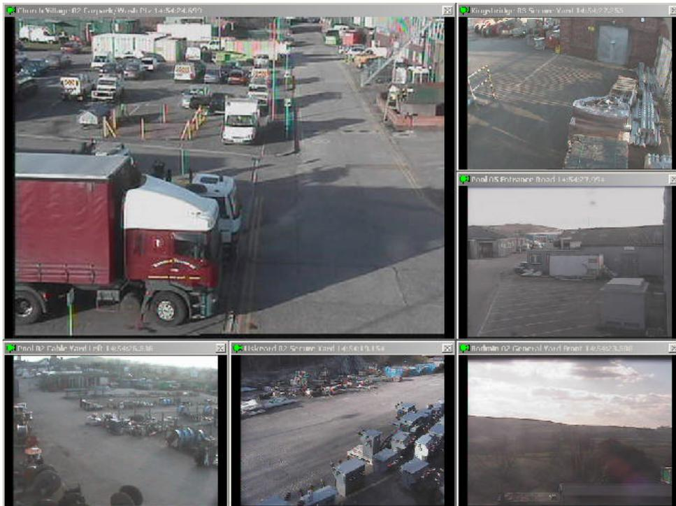
This screen picture shows a 6-view screen on a single monitor, each view is labelled with camera location, time of view and an icon showing alarm status.
