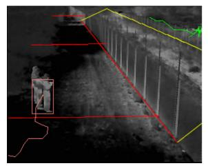
Fence lines can be monitored by multiple technologies, including; motion detectors attached to fences, microphones, TI cameras and standard visual spectrum cameras. In this picture 'virtual sensors' (the red and yellow lines placed in the image) are used to locate and track people by a visual intelligence system.
