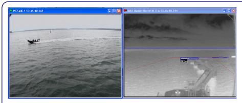
Using MIST's detection and tracking capability along with its flexible virtual sensors, ranger is able to provide the operator with up to date target position information as it moves through the field of view. All Ranger's geometry information is saved to disk along with the video data making it available for event review or for submission as evidence.
